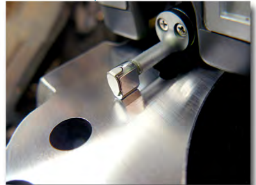
Profilometer stylus measures block surface
