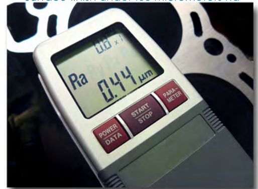
Surface finish under .50 micrometers Ra
